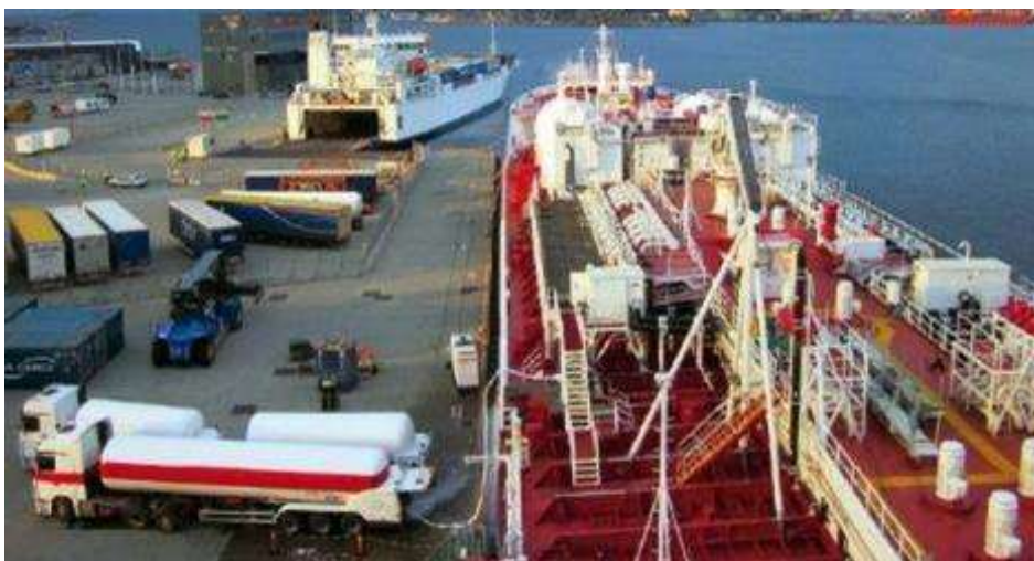
Figure 12 Truck to Ship LNG bunkering
