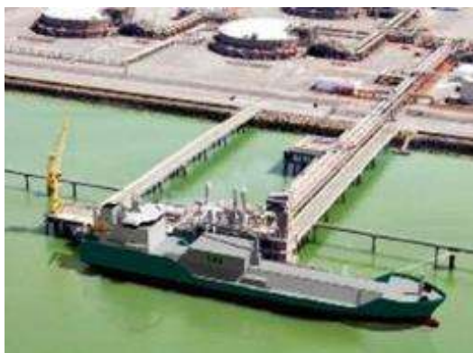
Figure 13 Shore to ship LNG bunkering
