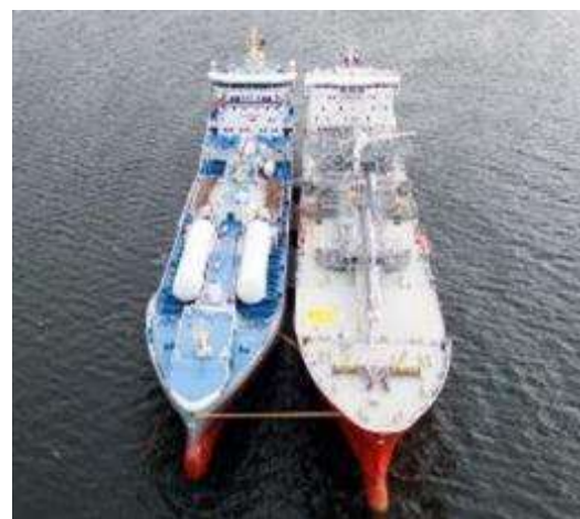
Figure 11 Ship to ship LNG bunkering
